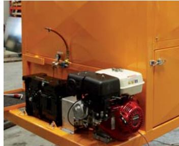
9 HP Honda engine for direct drive of auger (for AF 25 only)
