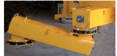
External conveyer auger has chute, insulation and remote control of discharge auger
