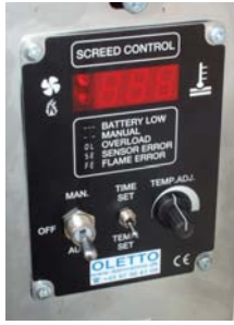
Computerized control of heating
