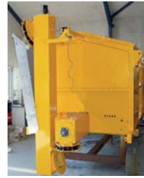
External conveyer auger in transport position
