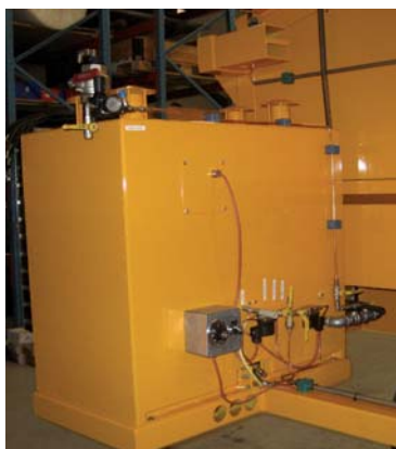
Built-in bonding agent (tack tar) tank
